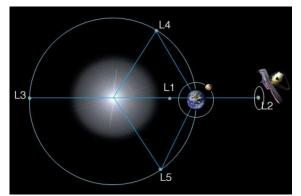
required for a small object to move with them. The L1, L2, and L3 points are all in line with each other - and L4 and L5 are at the points of equilateral triangles.
